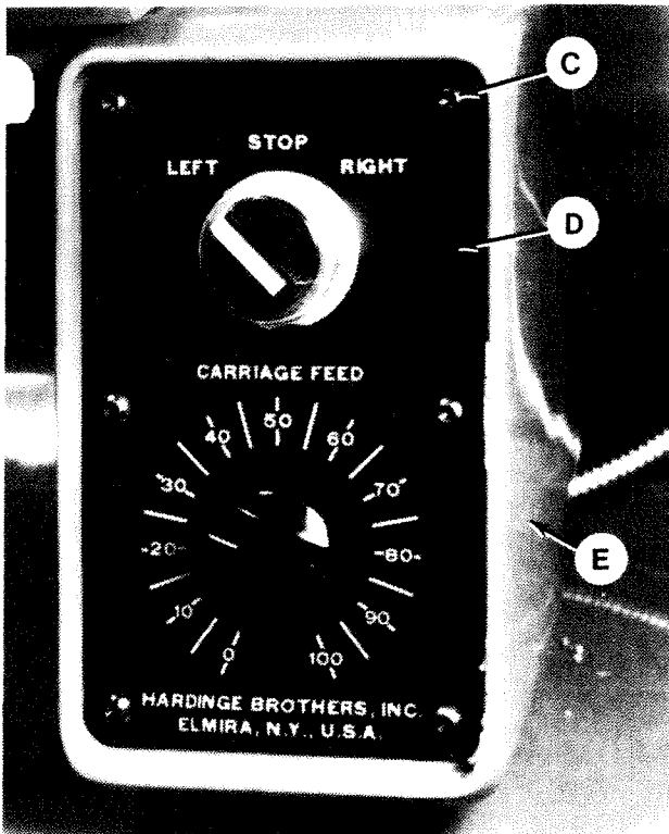
Figure 5.5 - Power Feed Control Panel (Front View)
